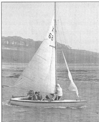
The 'Patsy', Tom and Trichia Gilmour's boat. Originally a 'Scow' type boat. Jimmy Longley rebuilt her, extending the bow forward from the mast position, and fitting a massive metal centreplate.
